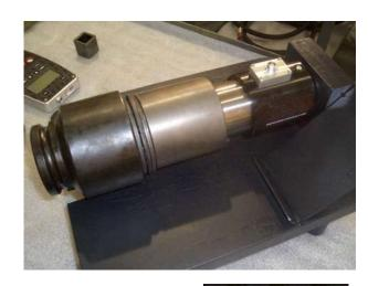
3. Connect the cable aligning the red dots on the cable with the red markings on the display and transducer.
