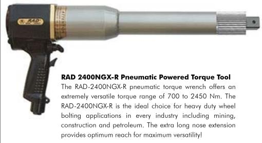
RAD 2400NGX-R Wheel Nut Bolting Series Torque Tool
